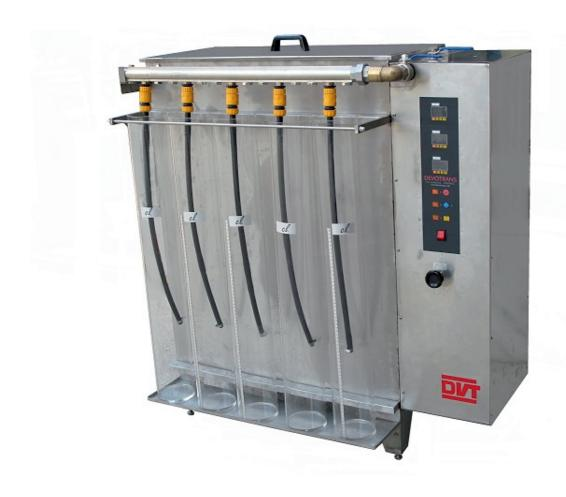
ENABLES TO CONDUCT LIFETIME TESTS UNDER PRESSURE FOR DROP BY DROP IRRIGATION PIPES
